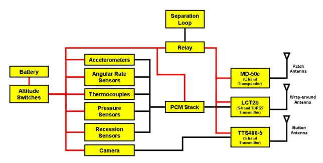
Figure 2. SCRAMP Block Diagram
