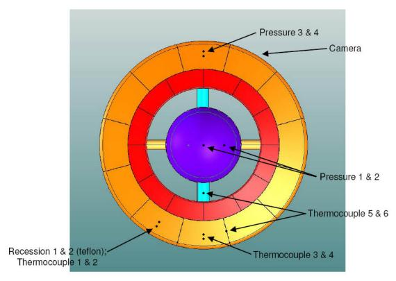
Figure 3. External Sensor Placement
