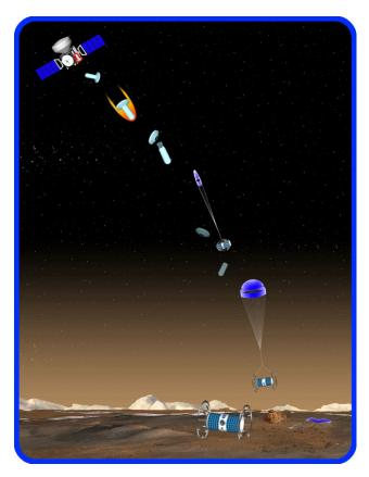
Figure 1. Atromos mission sequence (S/C separation, entry, descent and landing).
